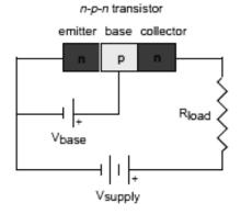
The voltage applied to the base is called the *base bias voltage*. If it is positive, electrons in the emitter are attracted onto the base. Since the base is very thin (approximately 1 micron), most of the electrons in the emitter flow across into the collector, which is maintained at a positive voltage. A relatively large current,  $I_{\rm C}$ , flows between collector and emitter and a much smaller current,  $I_{\rm B}$ , flows through the base.
