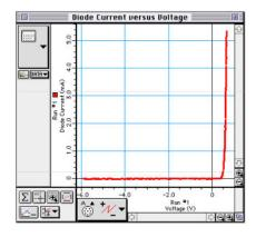
The vertical axis shows the current in milliamperes based on a calculation using the voltage drop across the 1 k $\Omega$  resistor. The horizontal axis shows Voltage across the diode.
