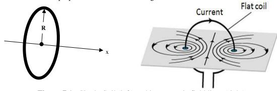
Figure 7.1: Single Coil (left) and its magnetic field lines (right)
