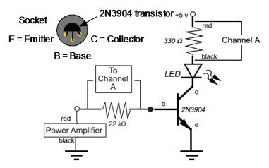
npn Transistor as Digital Switch
