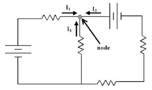
**Figure 4.1**: Current node in a circuit network
