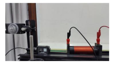
Figure 7.8: Solenoid Setup
