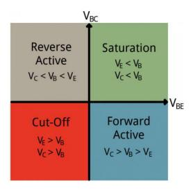
The simplified quadrant graph above shows how positive and negative voltages at those terminals affect the mode.
