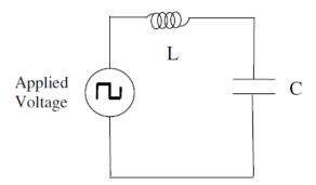
Figure 3.1: LC circuit
